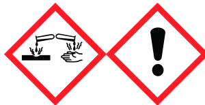
Corrosion Exclamation mark
