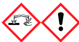
Corrosion Exclamation mark
