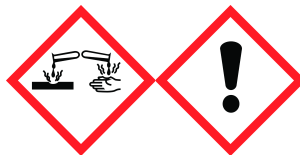
Corrosion Exclamation mark
