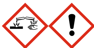
Corrosion Exclamation mark
